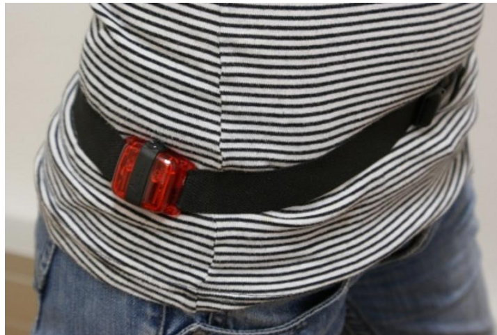
Figure 2. Picture of an accelerometer model, ActiGraph GT3X+, used in Kan2 survey (2014-2015).
