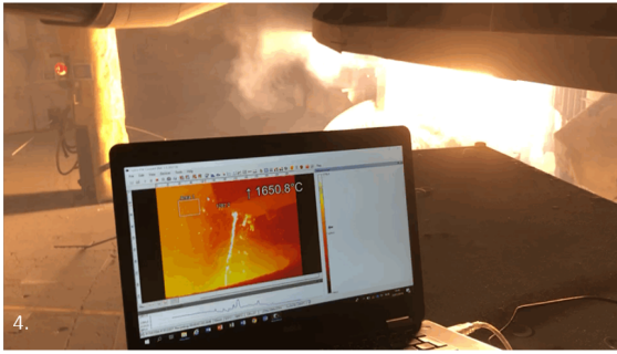
Figure 1.3: IR camera installed at Elkem Thamshavn oven nr. 2 [6].
