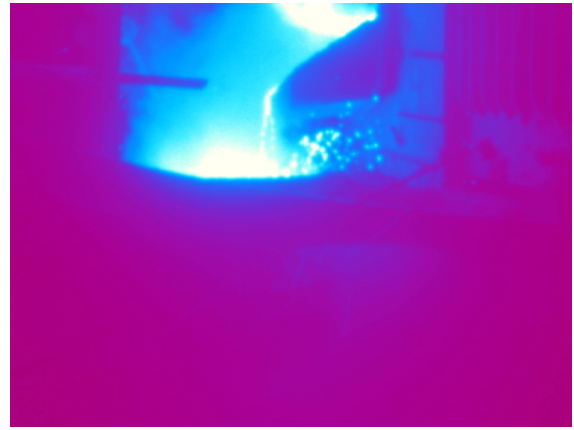
Figure 1.4: Thermal image from the tapping beam at Elkem Thamshavn oven nr. 2 [6].
