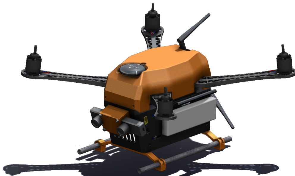
Figure 3.38: Drone design complete assembly
