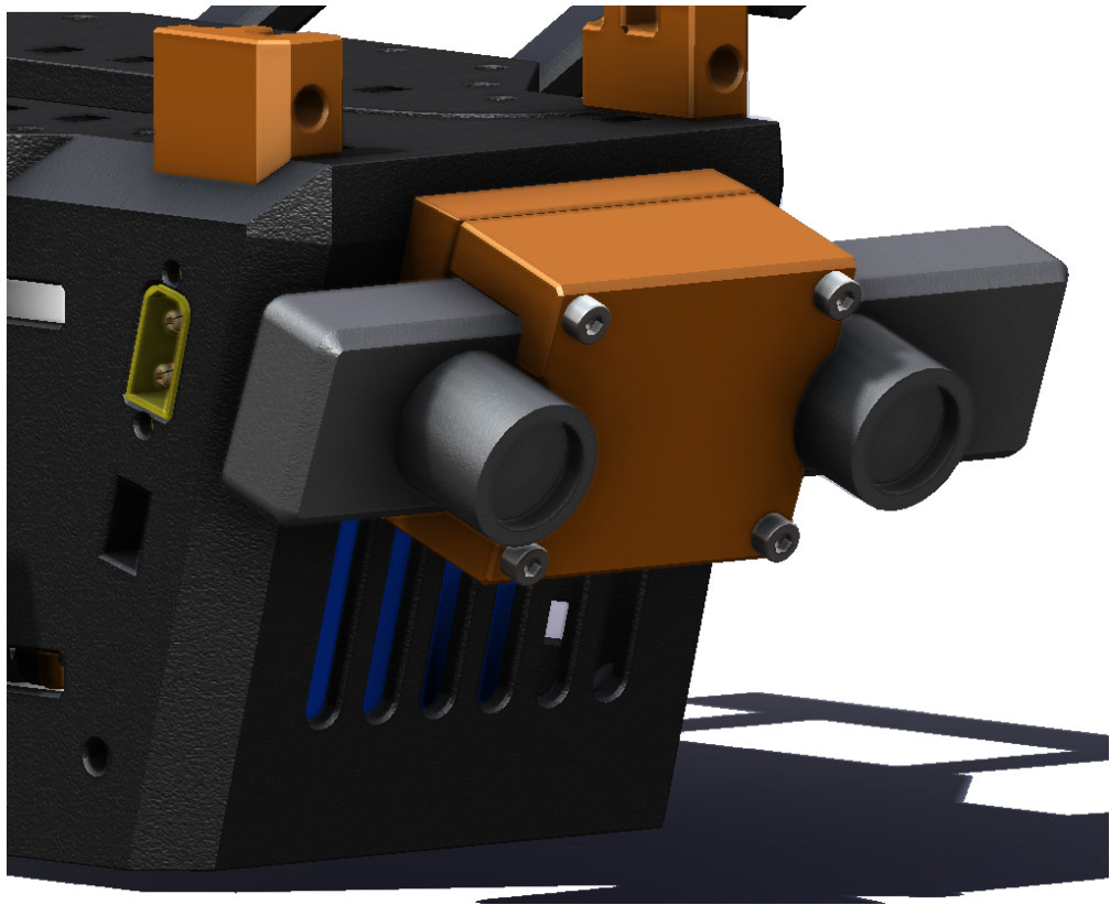
Figure 3.34: Drone design Zed Mini stereo camera mount
