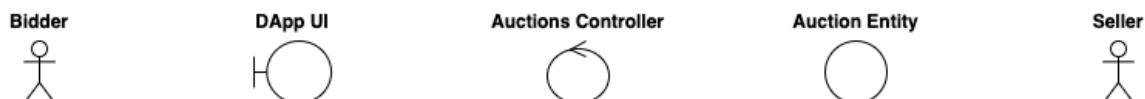
Figure 4.2: UML-symbols of the actors and components included in the Smart Trading Platform implementation
