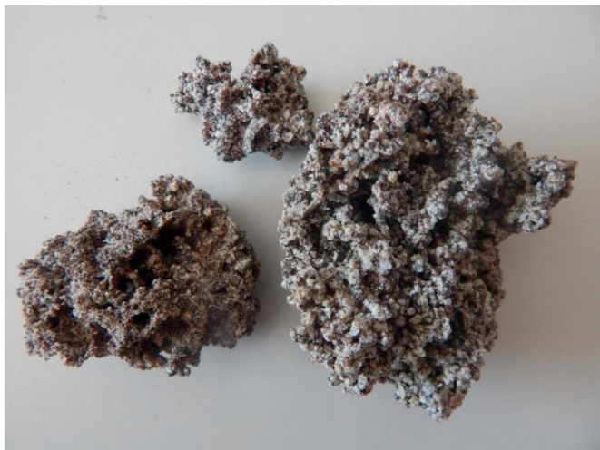
Fig. 14. Formation of agglomerates during grass pellet gasification.
