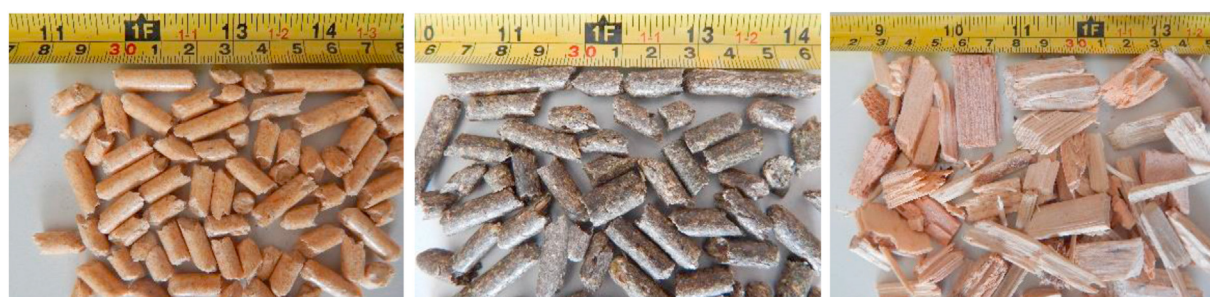
Fig. 3. Size range of wood pellets, grass pellets and wood chips.
