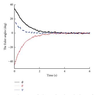
FIGURE 4: The response of Euler attitude angles in the absence of external disturbances.
