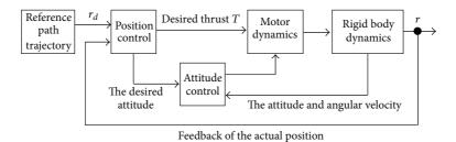
FIGURE 2: The control structure of the quadrotor UAV.
