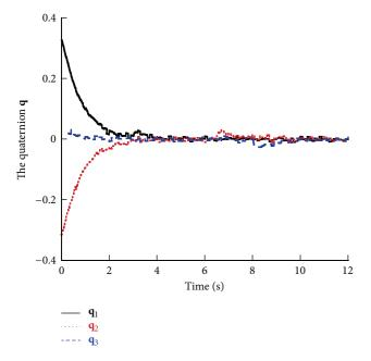
Figure 6: The response of the unit quaternion  ${\bf q}$  in the presence of external disturbances.
