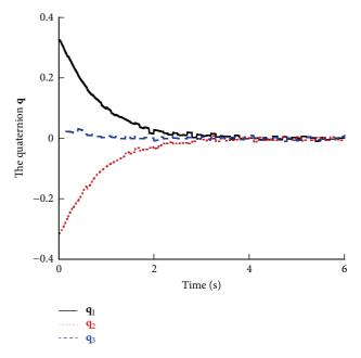
Figure 3: The response of the unit quaternion  ${\bf q}$  in the absence of external disturbances.
