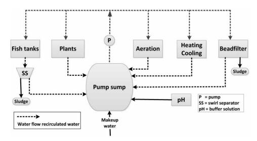
**Figure 1.** Flowchart of one of the two identical units of the aquaponic research facility showing water flows, water treatment, and sludge removal sites. The facility co-produced fish and vegetables with 100% recirculation of water.
