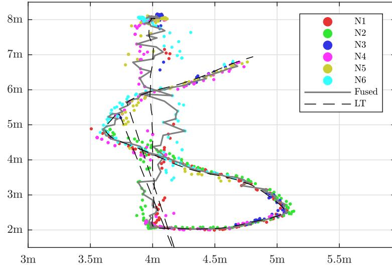
Figure D.14: Walked human path in XY plane at velocity 2.0 m/s using six sensor nodes N1-N6 and depth/YOLO (colored), averaged path (grey) and laser tracker.
