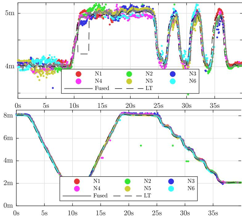
Figure D.12: Walked human path in the X-direction (top) and Y-direction (bottom) vs. time at velocity 1.0 m/s using six sensor nodes N1-N6 and depth/YOLO (colored), averaged path (grey) and laser tracker.
