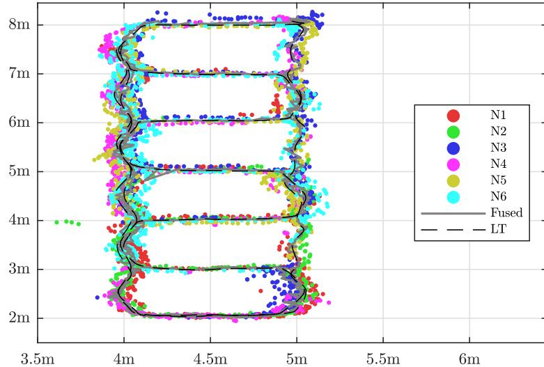
Figure D.8: Walked human path in XY plane at velocity 0.5 m/s using six sensor nodes N1-N6 and depth/YOLO (colored), averaged path (grey) and laser tracker.
