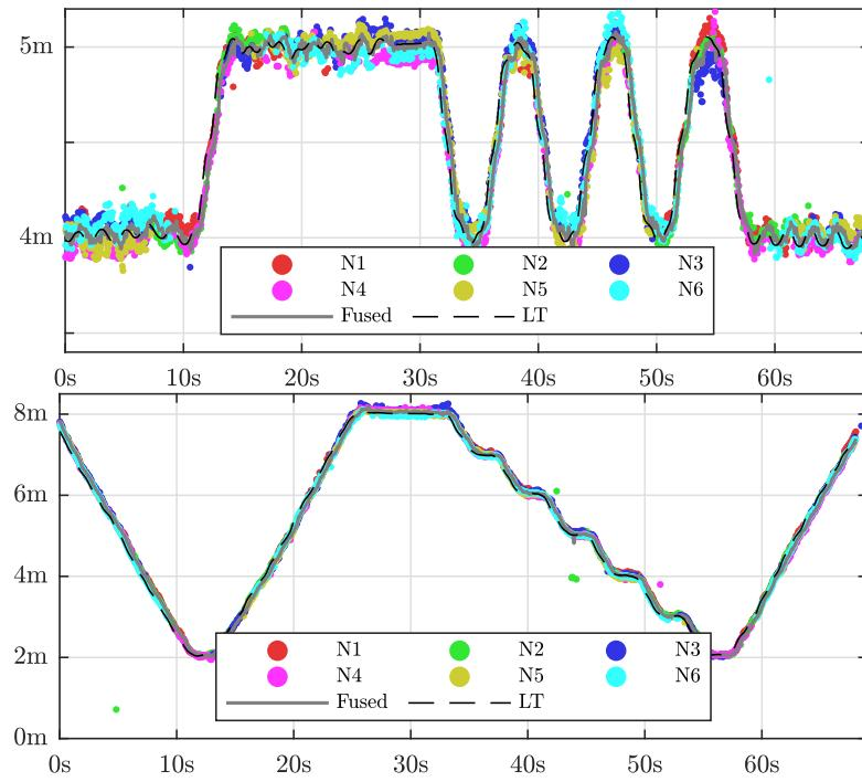
Figure D.9: Walked human path in the X-direction (top) and Y-direction (bottom) vs. time at velocity 0.5 m/s using six sensor nodes N1-N6 and depth/YOLO (colored), averaged path (grey) and laser tracker.
