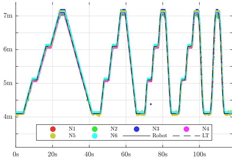
Figure D.4: Robot trajectory in Y-direction measured by the six sensors N1-N6, trajectory via robot and track resolvers and laser tracker.
