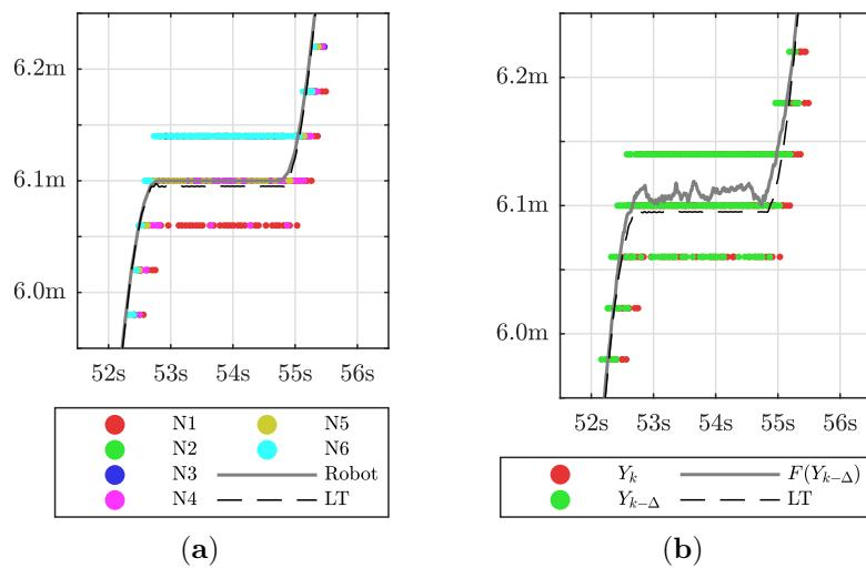
Figure D.5: (a) Selected section of Y-Position measured by 6 sensor nodes, robot position via resolvers and laser tracker. (b) Concatenated N1-N6 (red), the same with latency offset  $\Delta$  (green), concatenated and offset values with moving average filter (grey) and laser tracker (dashed).
