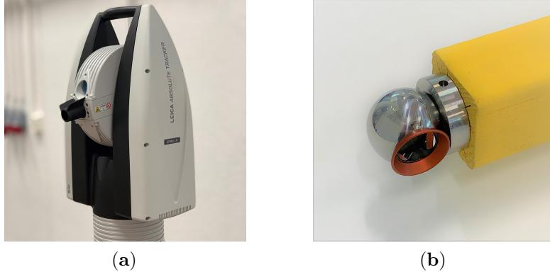
Figure D.3: Leica tracker AT960 (a) and Leica SMR Ball Probe (b)
