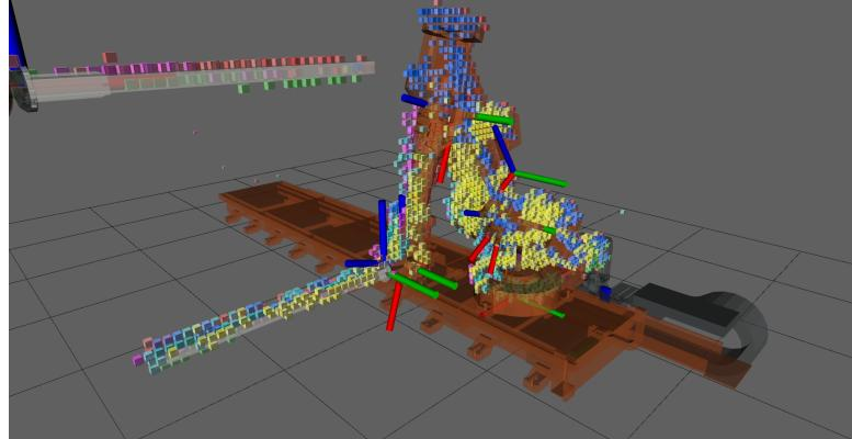
Figure D.6: 6 voxel maps overlaid on robot model at zero velocity.
