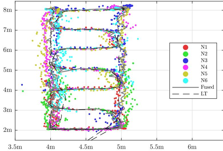
Figure D.11: Walked human path in XY plane at velocity 1.0 m/s using six sensor nodes N1-N6 and depth/YOLO (colored), averaged path (grey) and laser tracker.
