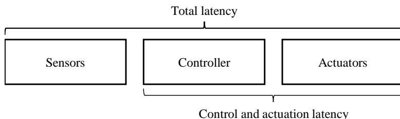
Figure D.1: Total latency in a control system including sensors, controller and actuators.
