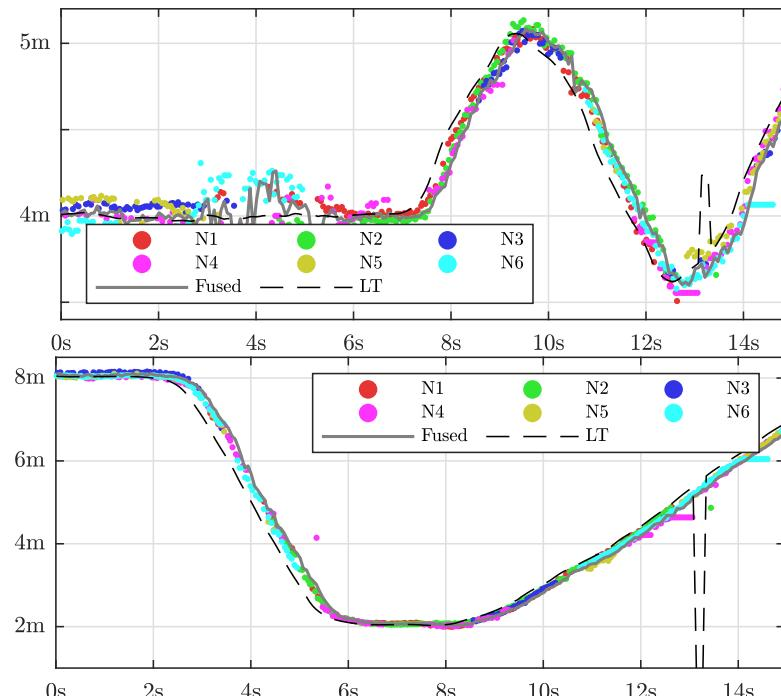
Figure D.15: Walked human path in the X-direction (top) and Y-direction (bottom) vs. time at velocity 2.0 m/s using six sensor nodes N1-N6 and depth/YOLO (colored), averaged path (grey) and laser tracker.
