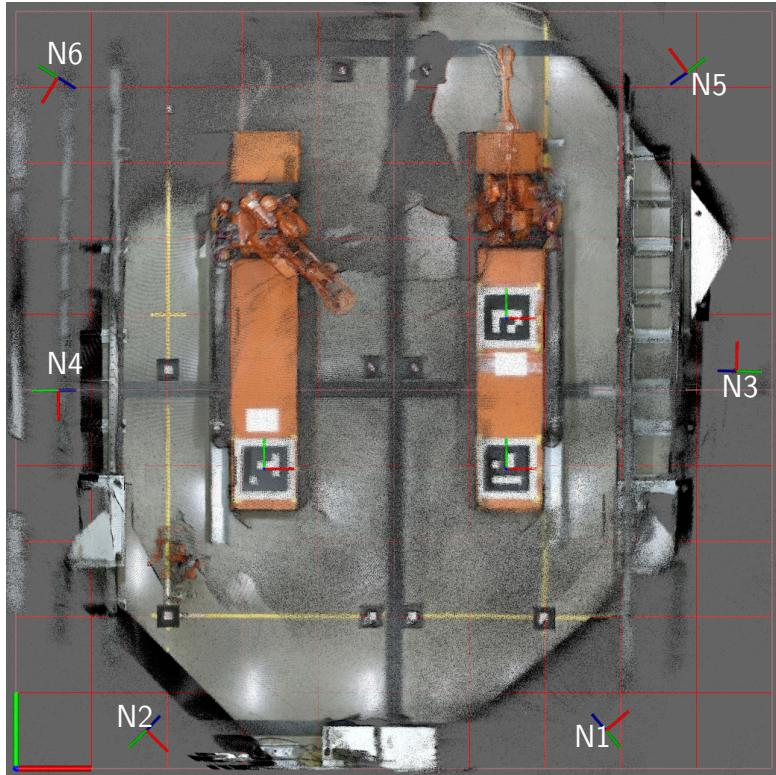
Figure D.2: Overhead view of the combined accumulated RGB point clouds of all six sensors after calibration. Sensor node poses are annotated N1-N6. The sensors are located 4.3 m above the floor and are angled approx. 60° from horizontal. The origin of the world frame is located at the bottom-left, where the red and green lines represent the X and Y-directions, respectively.
