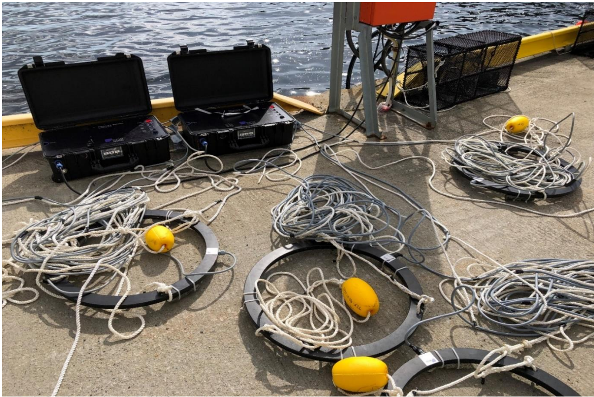
Figure 6. The circular antennas used in the study were deployed under water, lowered to the bottom, and tied to the pier with a rope. Each antenna covered specific stations at a particular time and detected the tagged fish passing over it. Photo: Özge Işın Starbatty.
