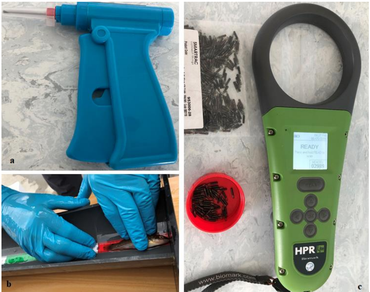
Figure 5. A PIT-tag injector (a), a goldsinny measured with an edged measuring device (b), half duplex PIT-tags and a PIT-tag reader (c). Photo: Özge Işın Starbatty.
