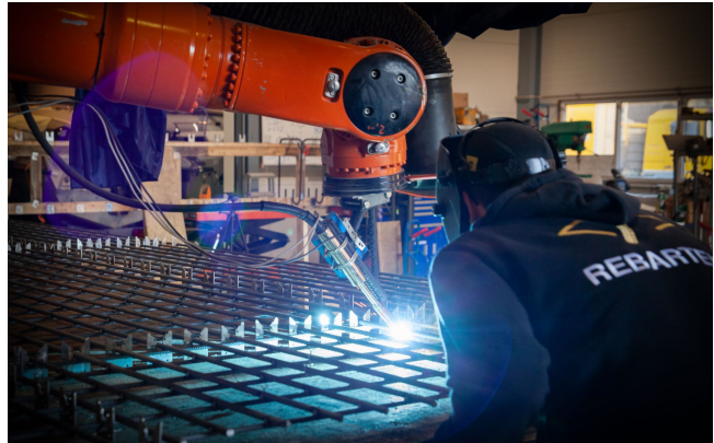
Figure 2.3 – Robotic fabrication method [12].
