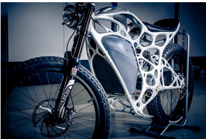
Figure 1.1 – The Light Rider motorcycle, by Altair and APWorks with 30% weight reduction [1].
