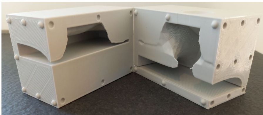
Figure 7.21 – 3D printed formwork: Vertical cut [Appendix C].
