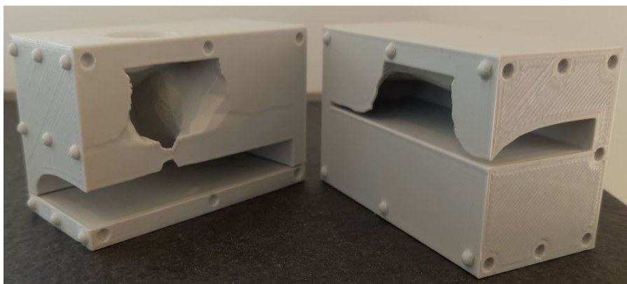
Figure 7.22 – 3D printed formwork: Vertical cut [Appendix C].
