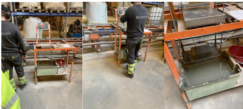
Figure 6.4 Density station and density procedure
