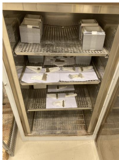
Figure 6.25 Drying cupboard and materials drying inside it
