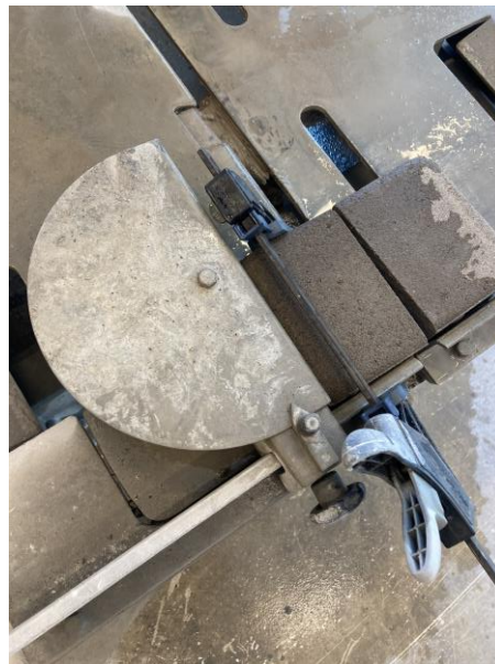
Figure 6.14 Clamp and metal disc for edge support
