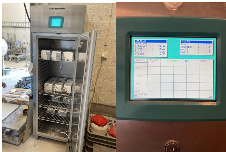
Figure 6.22 Placement inside chamber and starting details
