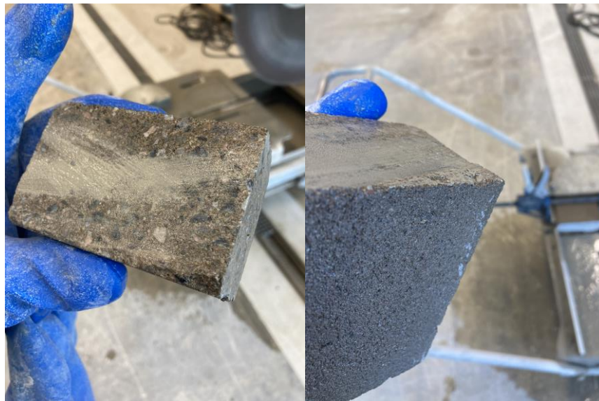
Figure 7.6 "free cement" and uneven cutting
