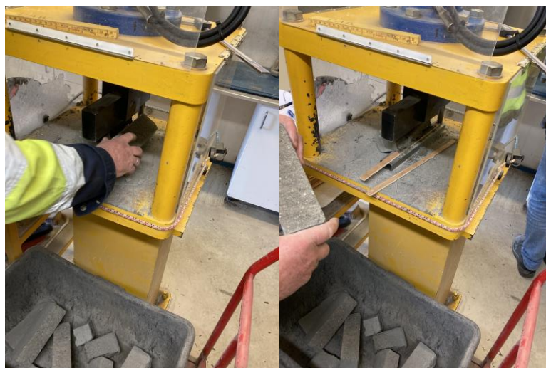
Figure 6.5 Tensile splitting strength machine at Aaltvedt Betong
