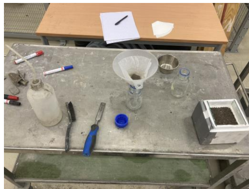
Figure 6.24 Filter paper, spray bottle and brush used to collect the scaled of material
