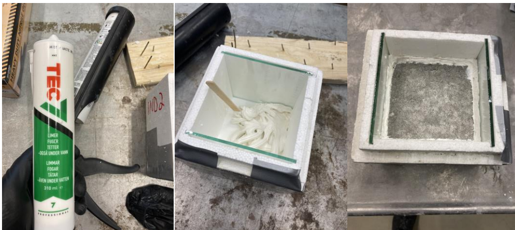
Figure 6.18 Tec7 and the fitting of the paving stones
