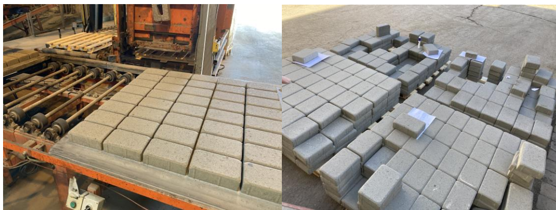
Figure 6.6 Stacking machine, pallets and pallets of cured SiGS paving stones
