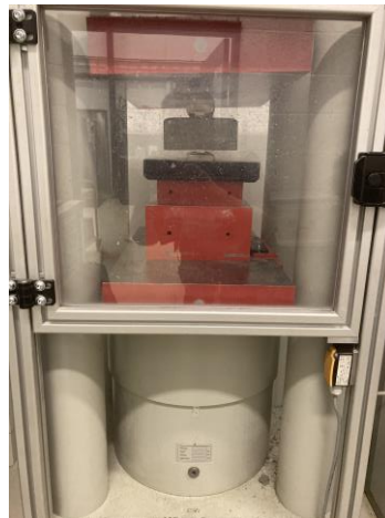
Figure 6.10 The setup in the UiA machine of the test of tensile splitting strength
