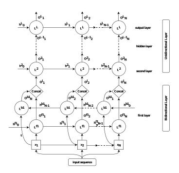
Fig. 1. Cascaded unidirectional and bidirectional LSTM-based DRNN model.
