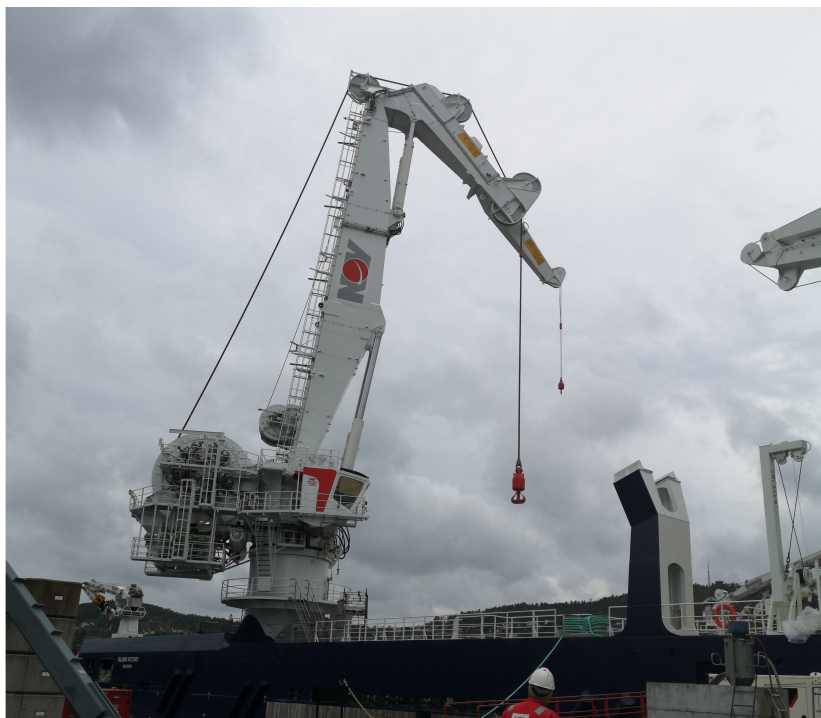
Figure 12. A 250t AHC crane from National Oilwell Varco placed on a vessel.
