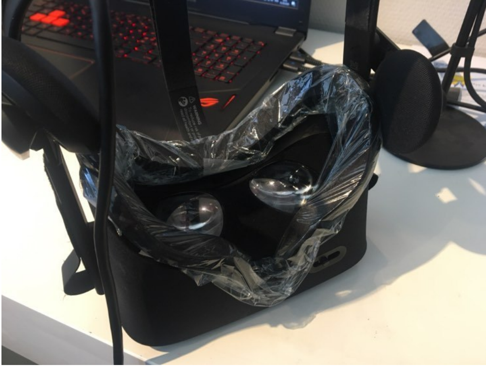
Figure 3.9: Oculus Rift with cling film.
