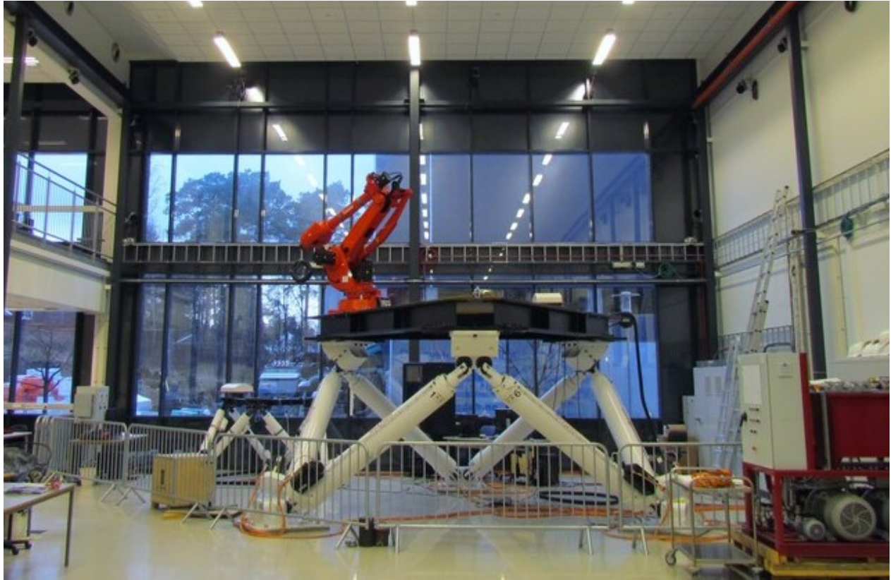
Figure 1.1: The two motion platforms at the Norwegian Motion Laboratory [8]. The smallest platform on the left is used for the biomechanics lab.
