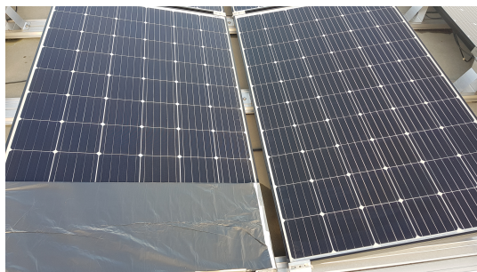
Figure 12: All three of module K5s substrings are covered
