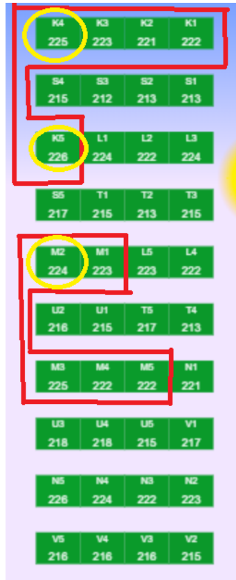
Figure 14: The various modules the experiments were conducted on and the strings they belong to. The modules circled in yellow are the covered modules.
