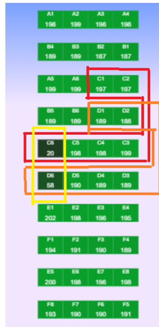
Figure 10: The two modules mostly afflicted by shade from the pyranometer and the string they belong to
