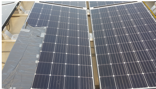
Figure 11: The plastic covers a part of one substring on module M2
