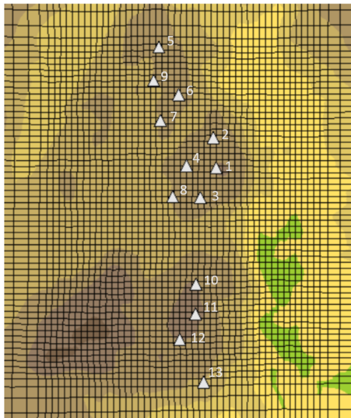
Figure 5.3: The placement of the wind turbines and how they are all inside the refinement area
