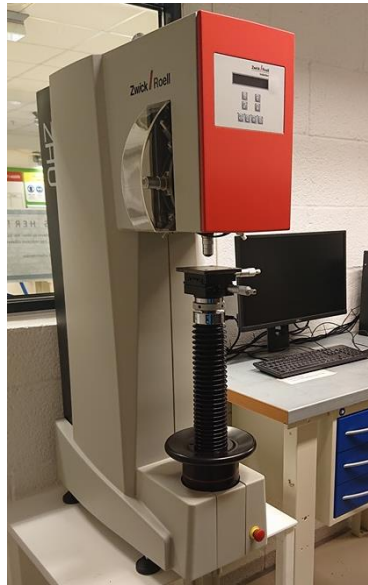
Figur 5.8: ZHU250CL Universal Hardness Tester
