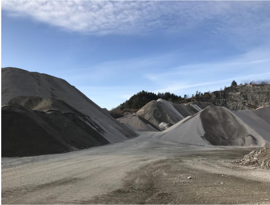
Figure 2: Piles and piles of the waste product from coarse crushed aggregate, crushed fine aggregate. Picture taken in Skien. [own]
