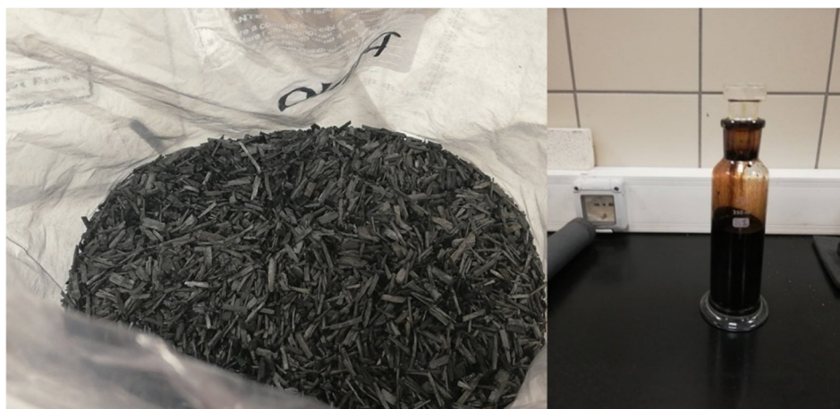
Fig. 6. Pine wood biocarbon (left); Pine wood pyrolysis oil (right) produced at University of Perugia, Italy.
