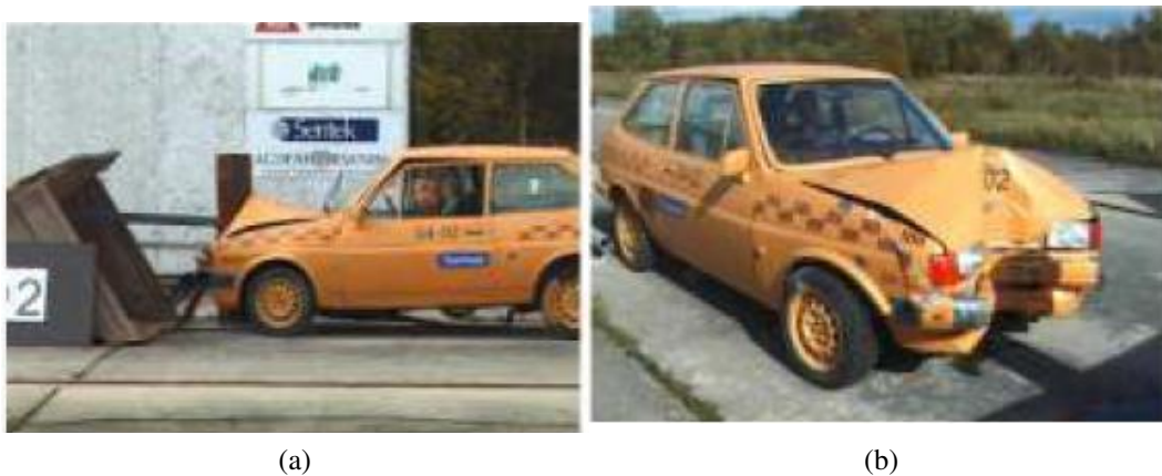
Figure 2.3: A full-scale frontal crash test of a standard Ford Fiesta 1.1 L 1987 model at 35 km/h, (a) Test vehicle during impact (b) Test vehicle after impact [70].
