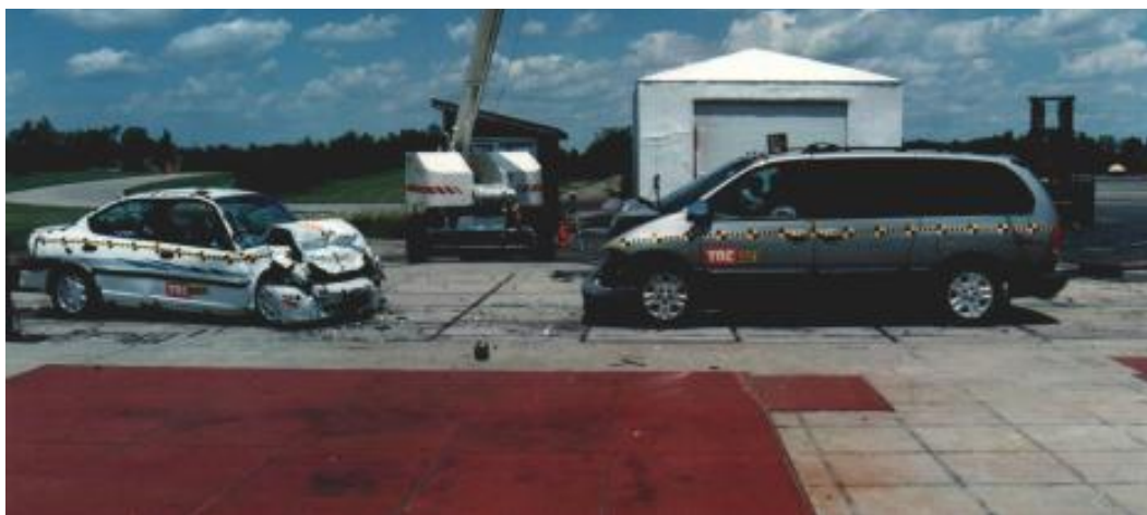
Figure D.1: Vehicles deformations after crash (Caravan left front-view, Neon right front-view)
