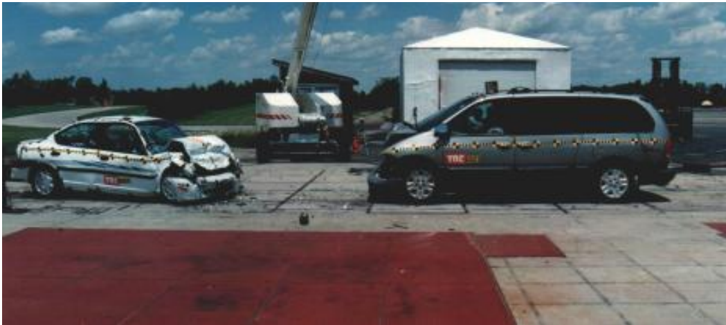
Figure 3.9: Vehicles deformations after crash (Caravan on right, Neon on left [1])
