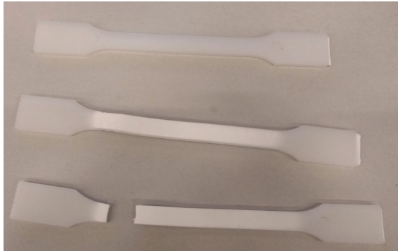
Figure 4.8: Result of tensile test with PP samples under high force (above sample for comparison).
