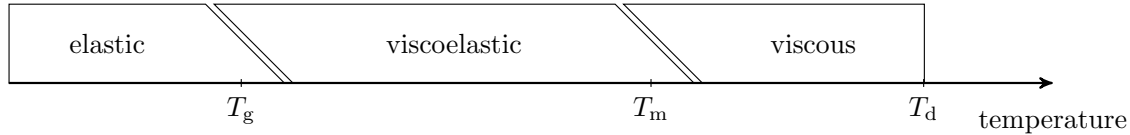
Figure 4.6: Behavior of semicrystalline thermoplastics at rising temperature [36].
