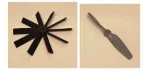
Fig. 8. Propellers: Left-low efficiency, Right-high efficiency
