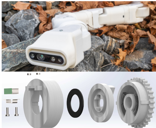
Fig. 1: Serpens , a low-cost snake robot with series elastic actuator (SEA), precision torque control and a screw-less assembly mechanism (top); the proposed design of the elastic gears for Serpens (bottom).
