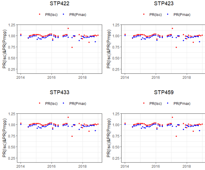
Fig. 6. Normalized module monthly PR with respect to P_{MPP} and I_{SC} .
