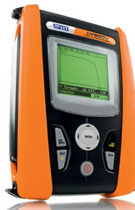
Figure 28: Shows the IV-curve tracer used for IV analysis [35]
