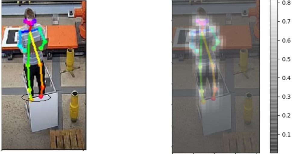
Figure 5.5: Resulting detection and confidence map in fake foot test, fake ankles circled
