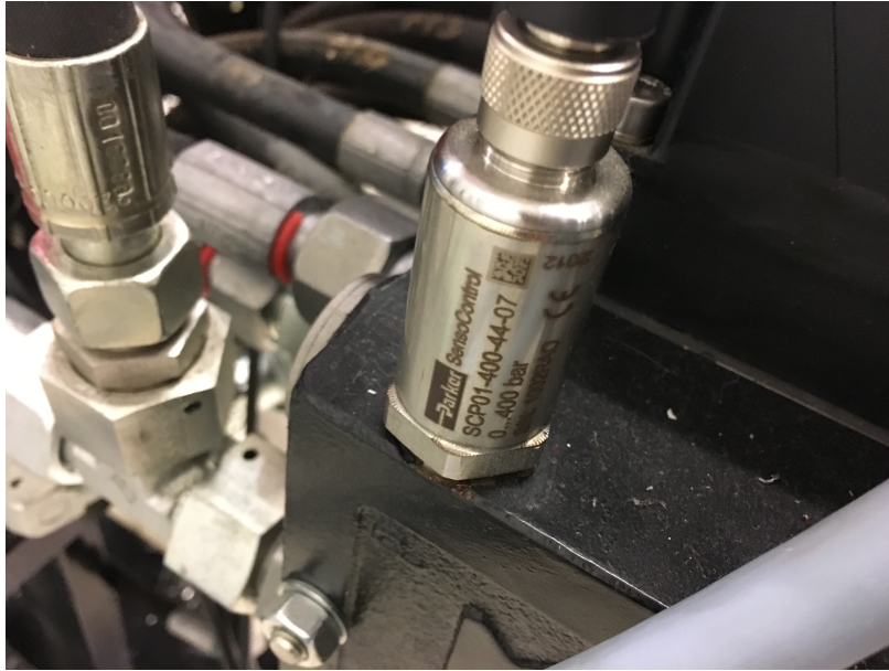
Figure 3.9: Parker SCP01 pressure sensor
