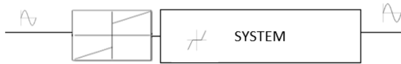
Figure 4.24: Open Loop State-Space Model
