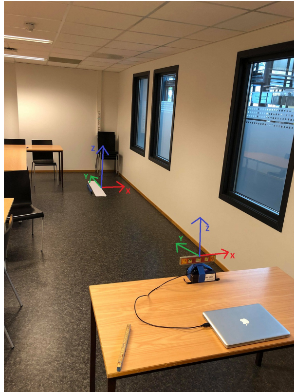
Figure 6.5: Coordinate System for Object and Camera
