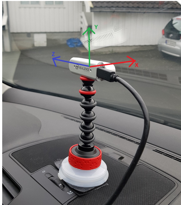
Figure 4.84: Cameras Coordinate System
