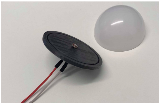
Figure 4.81: Diffuser Frame, Diffuser Dome and Photo Cell
