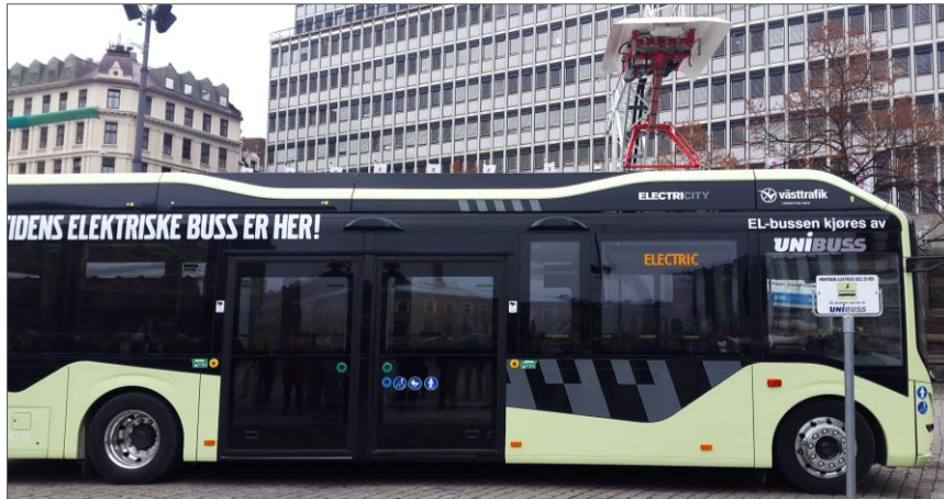
Figure 3. An electric bus in action of being charged by a pantograph station
