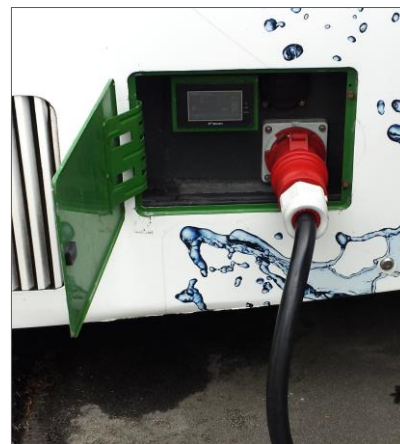
Figure 2. Conventional plug-in (43 kW)
