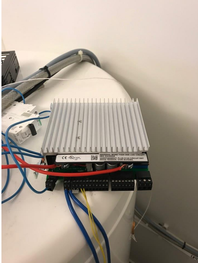
Figure 60 Thyristor during installation.
