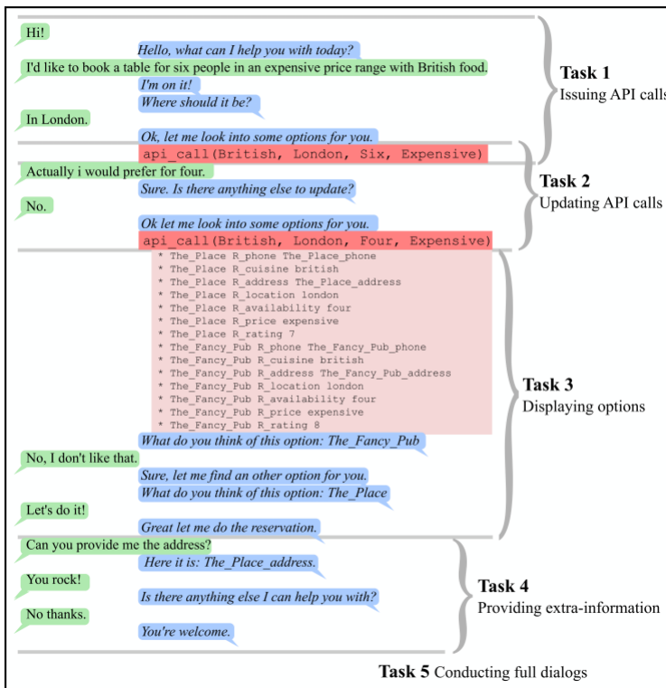
Figure 3.5: The different goal-oriented dialog tasks. A user (green) chats with a dialog system. Where the dialog system predicts responses (blue) and API calls (red), giving the API call results(light red) [16]
