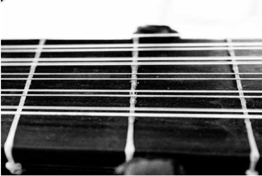
Figure 4.9. The frets are so worn out that they affect the sound by being too low. Small fragments sticking out also disturb the string's vibration. Photo: Robin Rolfhamre.
