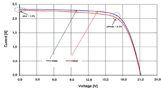
**Figure 3:** I-V Characteristics of normal and discolored PV modules [35].
