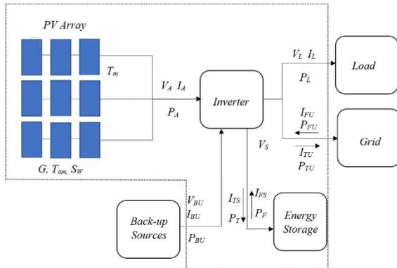
**Figure 4:** Diagram of basic real time parameters to be measured[57]
