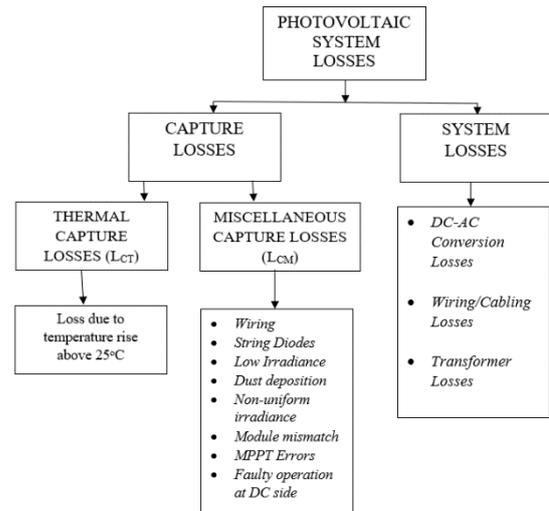
Figure 1: Categorization of losses in PV systems.
