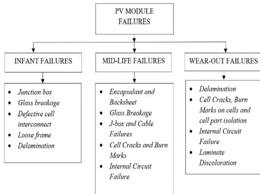
**Figure 2:** Major identified degradation modes of Crystalline PV modules [3]
