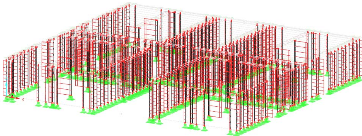
Figure B.15: Distribution of the internal normal forces in the studs of the first storey of the panel construction for LC1 (self-weight)
