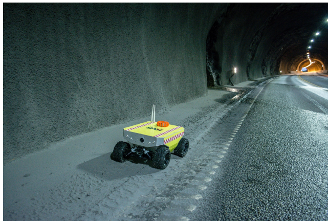
Figure 1.1: SPURV Responder robot in a tunnel [9]
