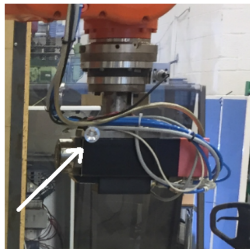
(b) Reflector Placement on Robot while Identifying Stiffness Joint 6
