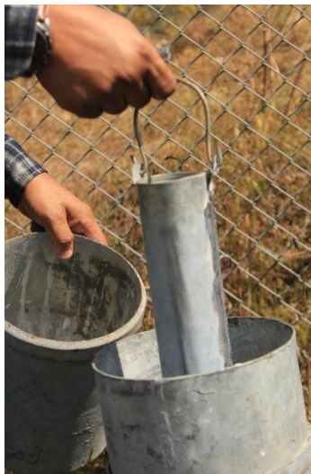
Figure 4.4: Manual Rainfall Measurement for the EWS
