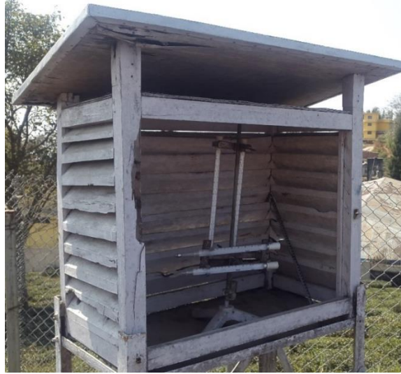
Figure 4.3: Manual Temperature Measurement for the EWS
