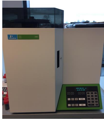
Figure A-1 PerkinElmer 2400 Series II CHNS/O Elemental Analyzer
