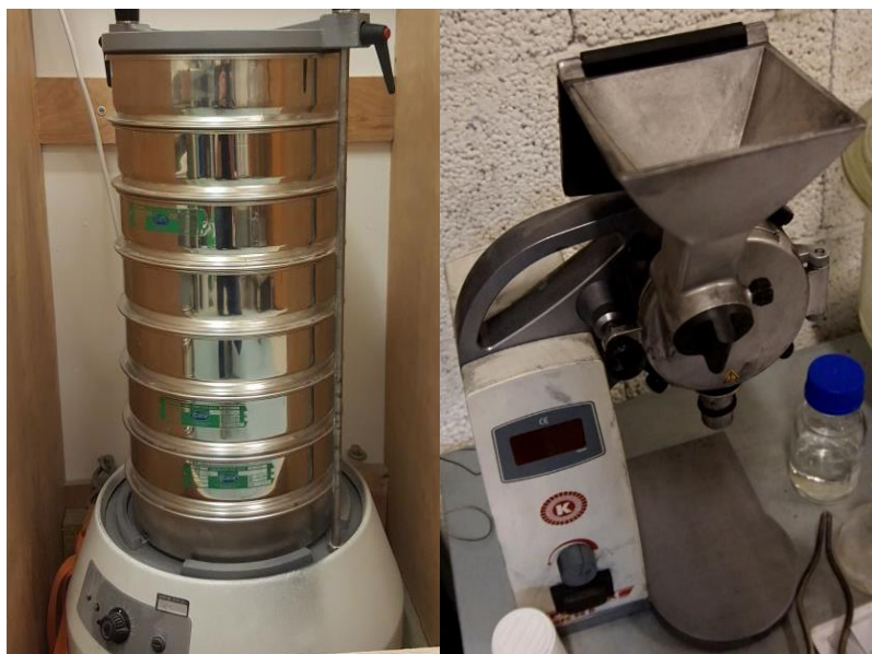
Figure 6-1: Left: Hammer mill with a 2 mm sieve. Right: Sieve analysis by sizes, (Gerrit Surup)
