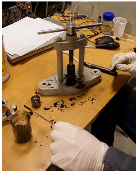
Figure 6-3: Manual pellet press (from bomb calorimetry)
