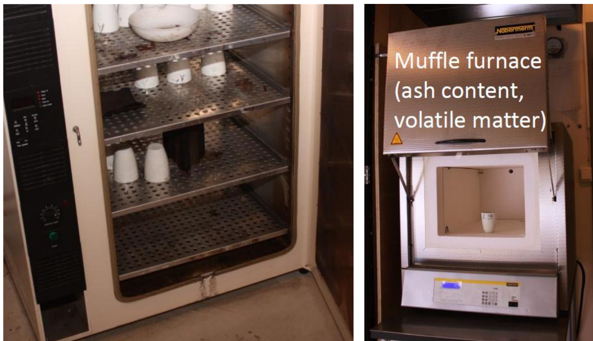
Figure 6-2: Left: Drying chamber (MC). Right: Muffle furnace (Henrik Kofoed Nielsen)
