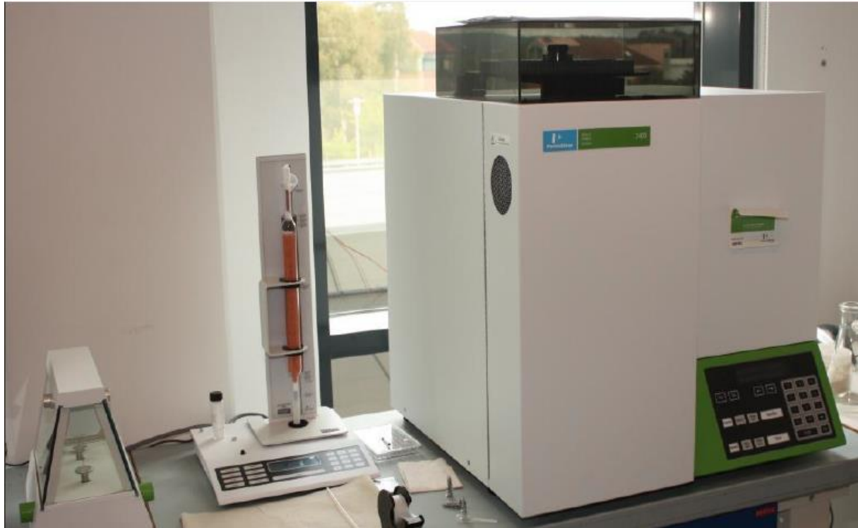
Figure 2-2: Elemental analysis with scale for ultimate analysis (Perkin Elmer 2400 CHNS/O Series II)
