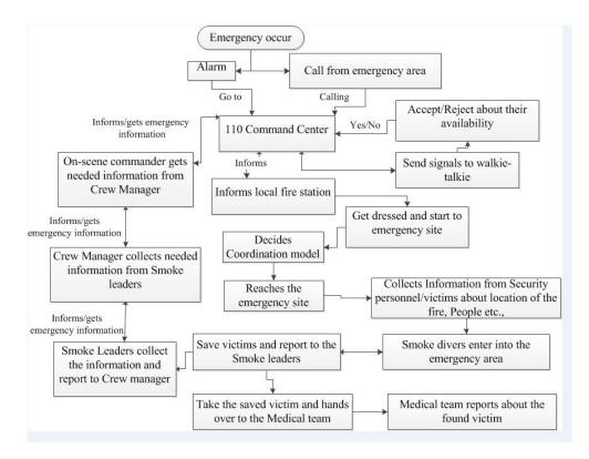
Figure D.1: Step-by-step Process of an Indoor Fire Emergency Response Operation
