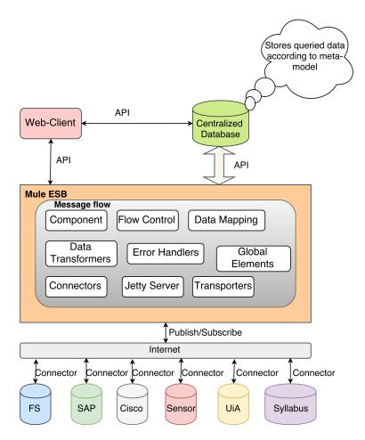
Figure C.2: A Data Integration Prototype for the Fire Emergency Response
