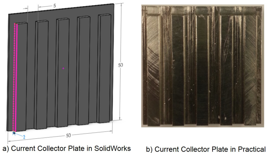
Figure 3.8: Current collector plate of the bipolar electrolysis stack
