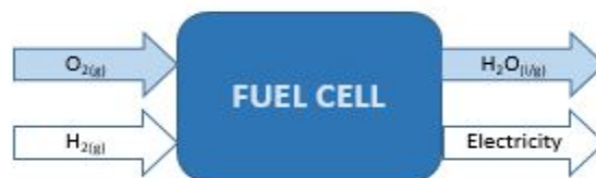
Figure 1.1: General overview of operation of fuel cell
