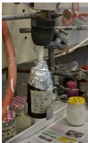
Figure 3.4: Mixing the chemicals using an electric mixer
