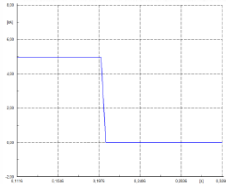
Figure 8. Current from PV at Node 1 during fault (current in kA versus time in sec).
