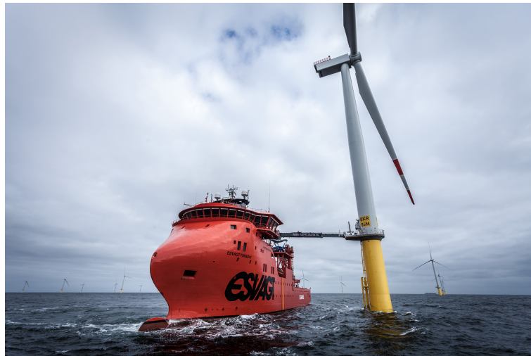
Figure 1.1: Example of an Offshore Access solution for payload transfer. Photo courtesy of Maersk.
