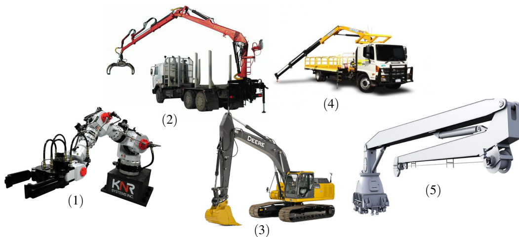
Figure 2.1: Hydraulic manipulators: Hydraulic robot (1) - Forestry machine (2) - Excavator (3) - Mobile crane (4) - Deck crane (5). (Photo courtesy of KNR System, Agrodetale, Deere, Rolls-Royce and Effer)
