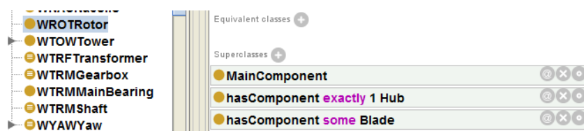
Figure B.8: Part-of relationship of WROTRotor class
