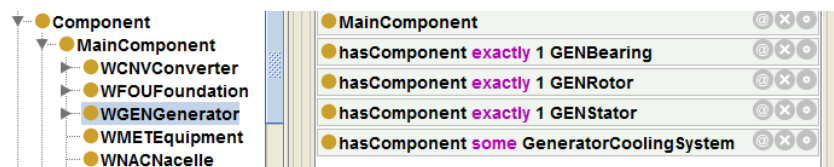
Figure B.12: WGENGenerator and its components
