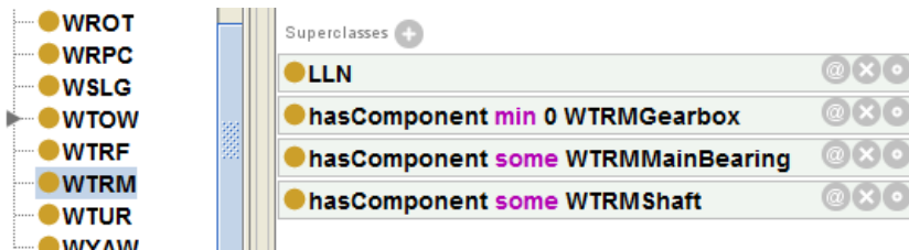
Figure B.9: Relationship between WTRM and its components
