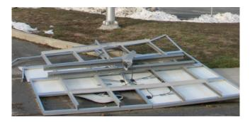
FIGURE 4.7: Illustrates PV modules that got destroyed during a storm [49].
