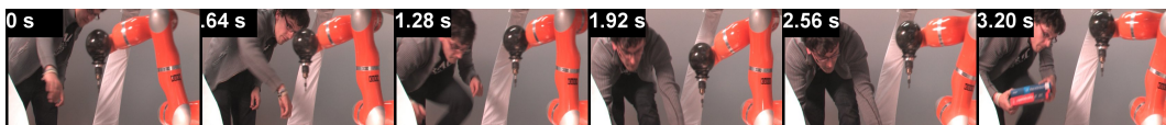
Figure D.9: Dynamic obstacle: A human worker enters the work area and the robot actively avoids him.
