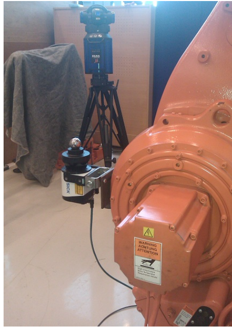
Figure B.3: FARO laser tracker used to calibrate the position of the laser scanner relative to the base of the robot.
