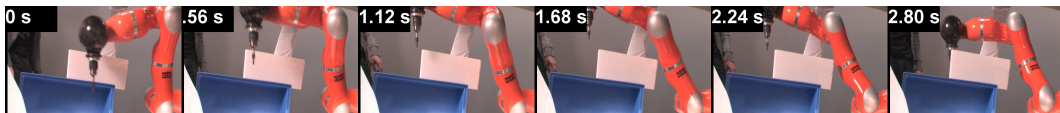
Figure D.8: Static obstacle: Another object is placed in front of the robot, to make the free movement volume even smaller.
