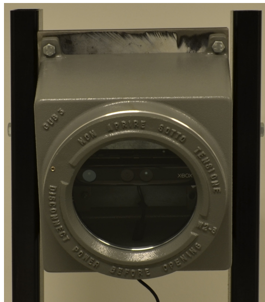
Figure E.3: The Microsoft Kinect mounted inside an explosion proof casing.
