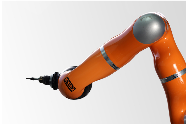
Figure D.1: The KUKA/DLR Lightweight Robot equipped with a chuck-tool, which enables the robot to conduct different operations equipping e.g. an umbraco bit or a bore bit.
