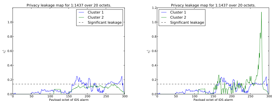
(a) Privacy leakage map for gzip compressed data. (b) Privacy leakage map for decompressed data.
