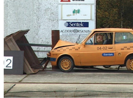
FIGURE 2: Vehicle undergoing deformation [19].
