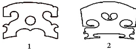
Typical Baroque (1) and Modern (2) bridge designs 11
